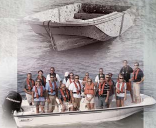
TOP: After taking 1000 rounds of .50-caliber bullets, a Whaler will still float.
